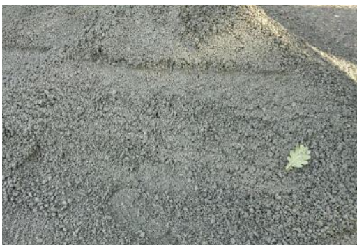
Crushed granite is particularly well suited as a bedding material
