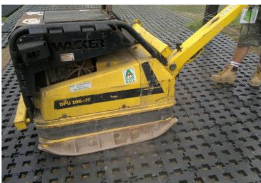
750 kg forward/reverse wacker plate
